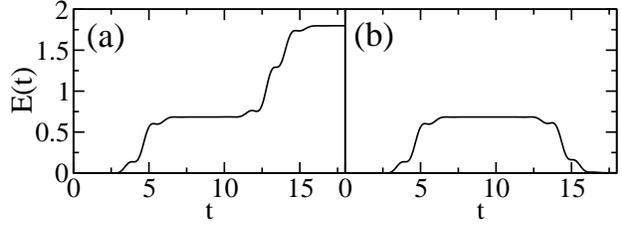
Fig. 2: The time-dependent energy expectation  $E(t)$  (measured from the lower level) for the Rabi model coupled with two successive pulses. Here, we take  $\epsilon = 1$ . Parameters for  $A(t)$ :  $A_0 = 0.5$ ,  $\omega_{\text{pump}} = 2\epsilon = 2$ ,  $t_d = 1$ ,  $t_1 = 4t_d$ . In (a),  $\Delta t = 3 \times \pi/\epsilon$ ; in (b)  $\Delta t = 3.5 \times \pi/\epsilon$ .
