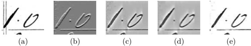
Figure 3: The five states of border removal using the Wiener filter (a-e). The original image (a), gradient image (in this case vertical) (b), gradient after deconvolution (c), median filtered deconvolution (d) and resulting image after scaling the intensity values (e).
