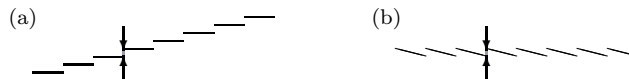
Figure 9: Spatial Fourier modes in a linear spatial structure with two degrees of freedom: piston and tilt. At low spatial frequency, a high-amplitude piston mode ( a ) gives the same ES signal as a low-amplitude tilt mode ( b ).
