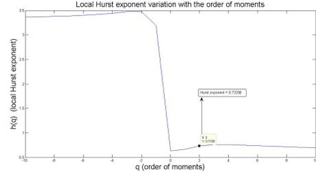
(b) The dependence of the generalized Hurst exponent  $h(q)$ , as a function of the order of the moment ( $q$ ), shown for  $V_0 = 40V$  and  $\omega = 70Hz$ , revealing the multi-fractal behavior.
