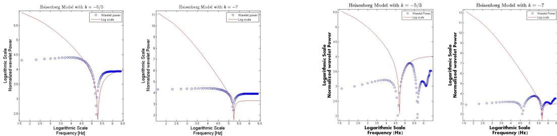
(a) Heisenberg fits for  $-\frac{5}{3}$  and  $-7$  exponents, shown for  $V_0 = 10V$  and  $\omega = 25Hz$ . (b) Heisenberg fits for  $-\frac{5}{3}$  and  $-7$  exponents, shown for  $V_0 = 10V$  and  $\omega = 100Hz$ .
