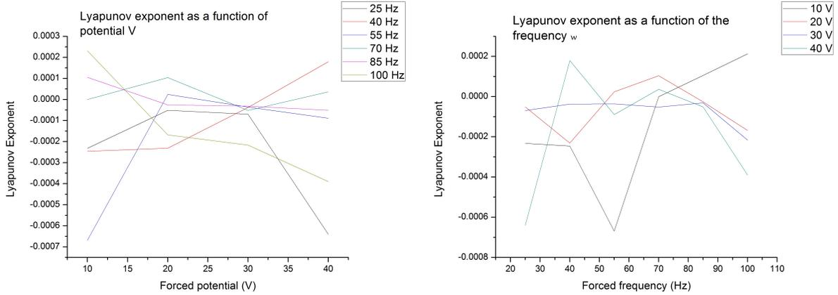
(a) Variations in the Lyapunov exponent as a function of forcing potential, for different frequency values. (b) Variations in the Lyapunov exponent as a function of forcing frequency, for different input potentials.
