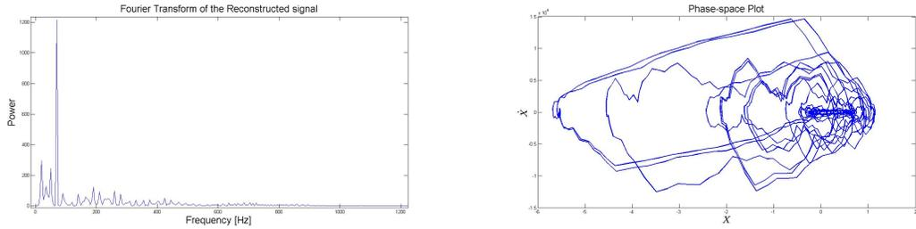
(a) The Fourier domain power spectrum of a typical signal. (b) Phase-space plot corresponding to the ‘Denoised’ version of the signal, clearly showing periodic motion.
