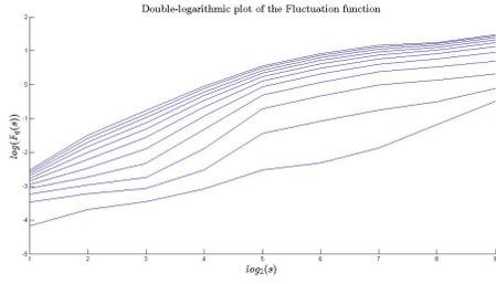
(a) Log-log plot of the fluctuation function  $F_q(s)$  vs. scale ( $s$ ) for various values of  $q$ , for the signal with  $V_0 = 40V$  and  $\omega = 70Hz$ .
