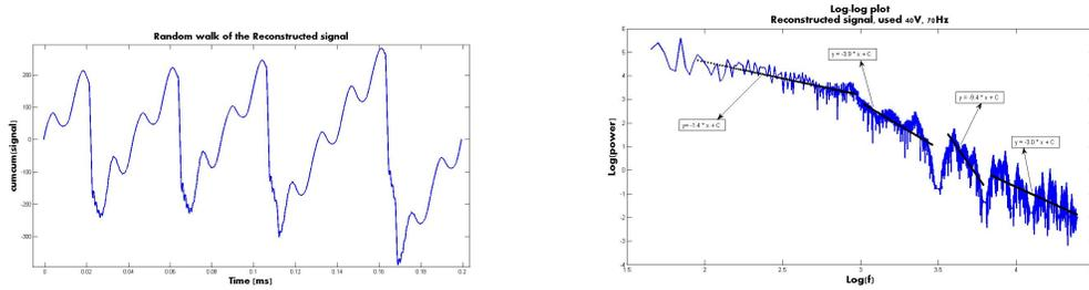
(a)Cumulative sum of the profile:  $y_i = \sum_{j=1}^i x_j$ . (b)Linear fit of the log-log plot of the Fourier power of the profile. In higher frequency domain, the Hurst exponent ( $H$ ) is found to be  $\approx 1$ , indicating extreme fractal.
