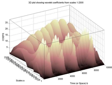
(a) 3D plot of the CWT coefficients with time and scale for  $40V$  and  $70Hz$  forcing parameters. Periodic behavior can be observed at certain scales.
