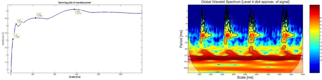
(a) Semilog plot of wavelet power, summed over all time at different scales. It is inferred that, the ball has periodicity of 18 ms, 49 ms, 226 ms and 578 ms corresponding to 40 V and 70 Hz forcing parameters. (b) Wavelet power spectrum with the cone of influence. The two dominant periods of the time series can be ascertained with the confidence level of 95%. Image colors are a representation of the Wavelet Power Spectrum (WPS) normalized by variance.
