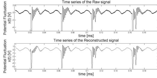
(a) Schematic illustration of the experimental setup. (b) A typical potential time series of the bouncing ball, with the corresponding denoised one shown below it, for forcing parameter values  $V_0 = 40V$  and  $\omega = 70Hz$ .
