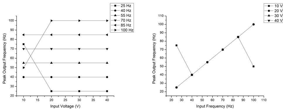
(a) Maximum output frequencies, shown for each input voltage to the system. Non-linear frequency response for 10 V input voltage is clearly seen. (b) Maximum output frequencies for different input frequencies, showing non-linear behavior for frequency values 25 and 100 Hz.
