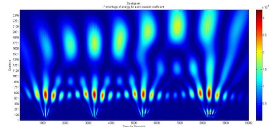
(b) Scalogram showing energy for each wavelet coefficients, with  $40V$  and  $70Hz$  as forcing parameters, clearly demonstrating the dominant periodic components.
