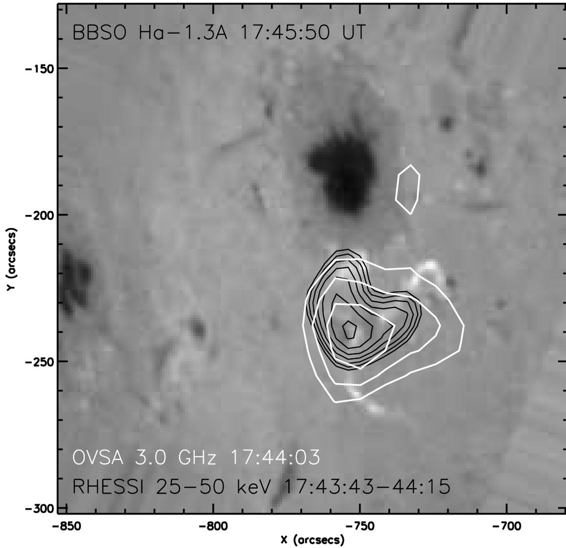
Fig. 2.— The 25-50 keV RHESSI source (black contours) and the OVSA microwave source (white contours) in comparison with the H $\alpha$  blue wing image (background greyscale image) from the BBSO. These images are chosen to be near one of the flare peak time 17:44 UT.
