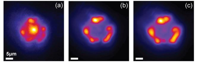
FIG. 9: The inner ring dependence on applied voltage. (a-c) The inner ring with increasing voltage:  $V_g = 1.5 \text{ V}$  (a),  $2.5 \text{ V}$  (b), and  $3.5 \text{ V}$  (c). The emission peak seen in the center of the ring is due to bulk GaAs emission in the spectral range of indirect excitons.  $P = 10 \mu\text{W}$ ,  $E = 1960 \text{ meV}$ .
