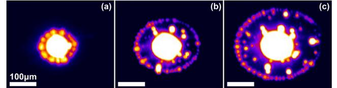
FIG. 10: The external ring dependence on excitation power. (a-c) The external ring with increasing excitation power:  $P = 310 \mu\text{W}$  (a),  $560 \mu\text{W}$  (b), and  $930 \mu\text{W}$  (c).  $V_g = 1.24 \text{ V}$ ,  $E = 1960 \text{ meV}$ .
