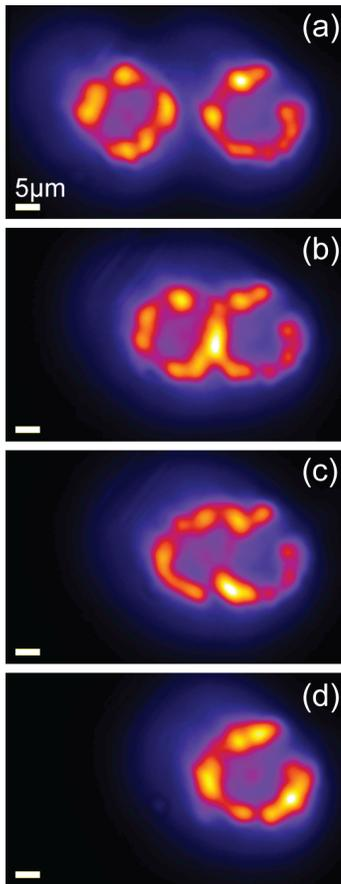
FIG. 12: Merging of two inner rings. (a-d) The emission pattern showing two inner rings created by two laser excitation spots merging into one spot as the left laser excitation spot is moved to the right. Laser power for both excitations  $P = 10 \mu\text{W}$ , applied voltage  $V_g = -3 \text{ V}$ .
