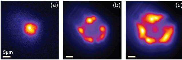
FIG. 8: The inner ring dependence on excitation power. (a-c) The inner ring with increasing excitation power:  $P = 4 \mu\text{W}$  (a),  $9 \mu\text{W}$  (b), and  $12 \mu\text{W}$  (c). The emission peak seen in the center of the ring in (b,c) is due to bulk GaAs emission in the spectral range of indirect excitons.  $V_g = 3 \text{ V}$ ,  $E = 1960 \text{ meV}$ .
