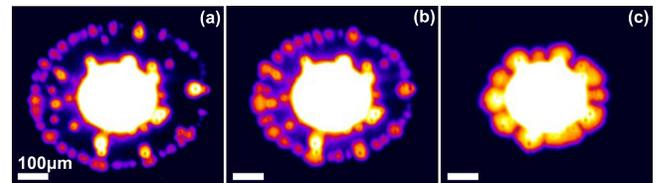
FIG. 11: The external ring dependence on applied voltage. (a-c) The external ring with increasing voltage:  $V_g = 1.262 \text{ V}$  (a),  $1.274 \text{ V}$  (b), and  $1.3 \text{ V}$  (c).  $P = 1400 \mu\text{W}$ ,  $E = 1960 \text{ meV}$ .
