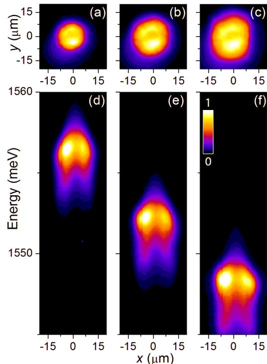
FIG. 7: Inner ring for a lower-energy Ti:Sapphire laser excitation. (a-c) Spatial images of the indirect exciton emission for the electrode voltage  $V_g = -2$  V (a),  $-2.5$  V (b), and  $-3$  V (c). (d-f)  $x$ -energy images of the indirect exciton emission for the electrode voltage  $V_g = -2$  V (d),  $-2.5$  V (e), and  $-3$  V (f). The laser excitation power  $P = 16 \mu\text{W}$  (a-c) and  $10 \mu\text{W}$  (d-f), and energy  $E = 1771$  meV.
