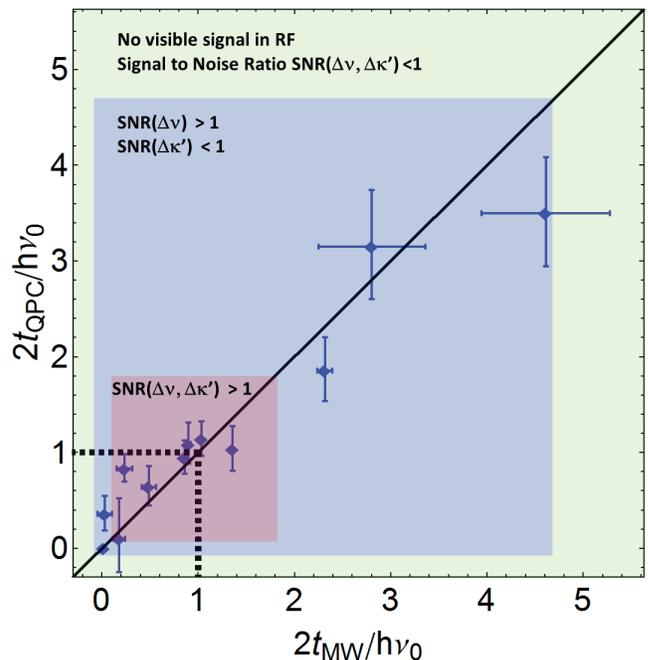
FIG. 5: (color online) Comparison of tunnel coupling extracted from QPC and microwave measurements. Colored regions highlight the  $2t/h\nu_0$  ranges over which  $\Delta\nu$  and  $\Delta\kappa'$  signals were observable. An observable signal corresponds to a signal-to-noise ratio  $\text{SNR} > 1$  when each point of the spectrum is acquired with an integration time  $\tau = 168$  ms.
