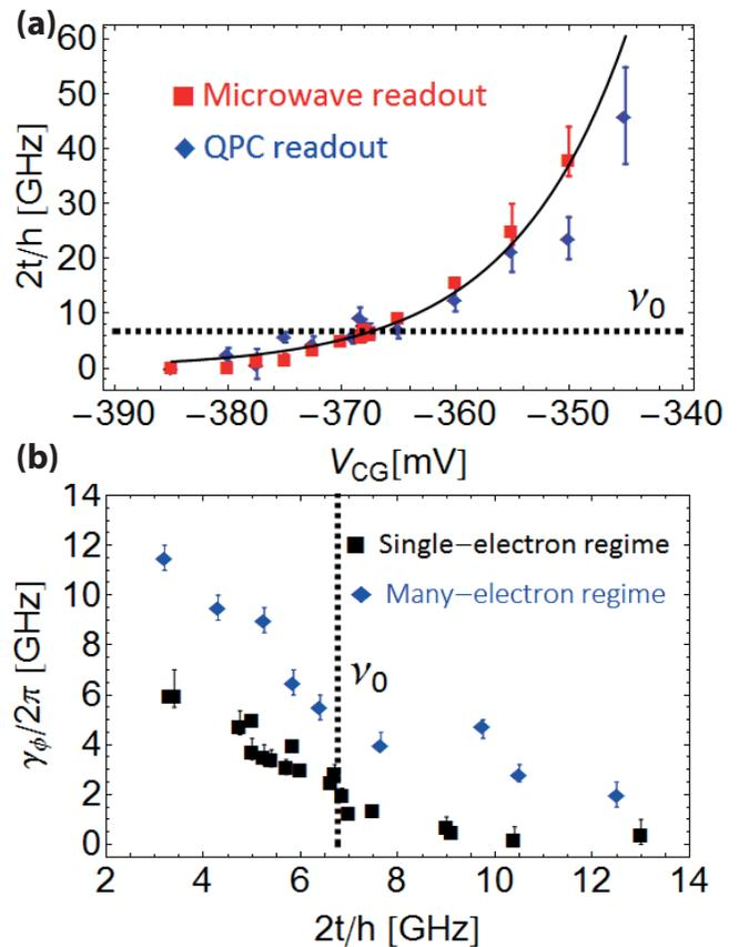
FIG. 4: (color online) (a) Tunneling rates  $2t/h$  between the dots measured vs  $V_{CG}$  for the two methods: charge detection with a QPC and microwave polarizability measurement. The black line corresponds to an exponential fit of  $t$  vs  $V_{CG}$ . (b) Dephasing rates  $\gamma_\phi/2\pi$  vs tunneling  $t$  in the single-electron and many-electron ( $\approx 50$  in each dot) regimes.
