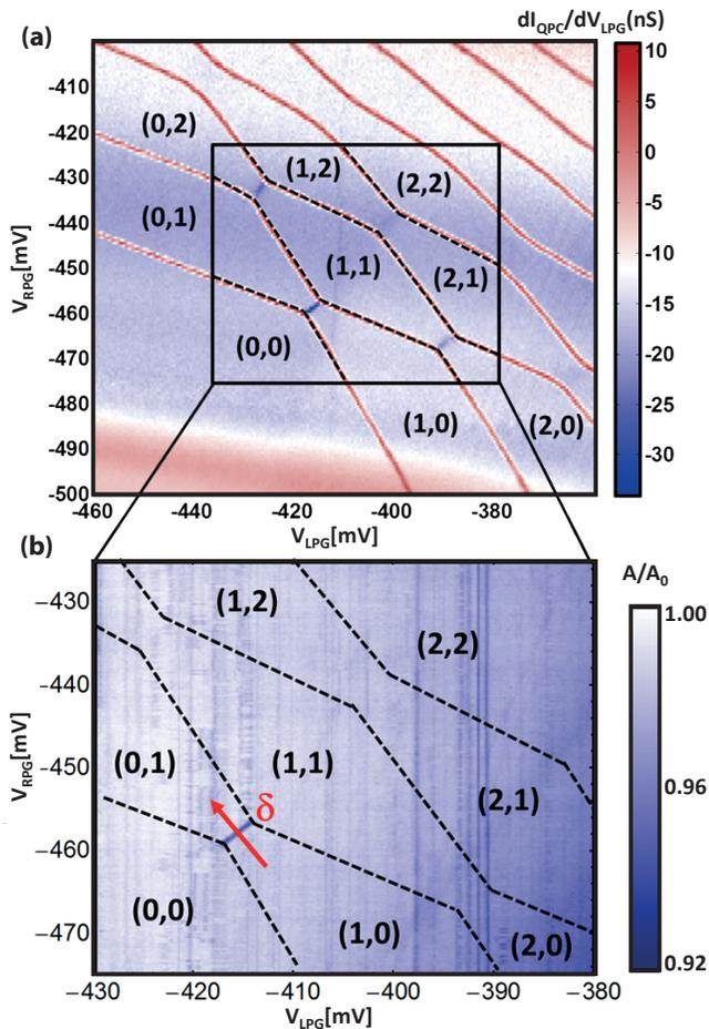
FIG. 2: (color online) (a) Transconductance  $dI_{\text{QPC}}/dV_{\text{LPG}}$  vs  $V_{\text{LPG}}$  and  $V_{\text{RPG}}$  obtained with the QPC. (b) Normalized transmitted amplitude through the resonator vs  $V_{\text{LPG}}$  and  $V_{\text{RPG}}$  in the range indicated in (a). In both cases, black dashed lines highlight boundaries between different charge states extracted from the measurement shown in (a).
