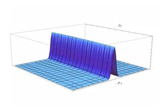
FIG. 2. Plot of Wigner function in the case with constant  $\gamma$  for  $|r_k| = 6.6$  and  $\gamma = 100$  showing high squeezing of a particular mode in the direction of momentum canonical to field variable
