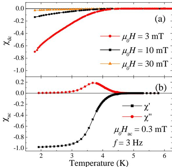
FIG. 2: (Color online). (a) Temperature dependence of the dc magnetic susceptibility of  $\text{Sn}_{0.6}\text{In}_{0.4}\text{Te}$  measured by zero-field-cooled warming (ZFCW). (b) Temperature dependence of the ac susceptibility of  $\text{Sn}_{0.6}\text{In}_{0.4}\text{Te}$  showing  $\chi'_{ac}$  and  $\chi''_{ac}$  through the superconducting transition. A demagnetization factor has been applied to account for the plate-like shape the sample [17].
