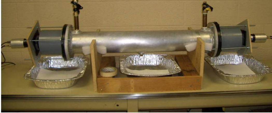
Fig. 1. The setup of our liquid scintillation detector. The aluminum foil pans are required for safety in case of leaks.
