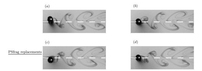
FIG. 2: Wake visualization during one cycle of oscillations of chain 2 for Re = 106. The white dashed line on each picture shows the location of the chain at rest. (a) and (c) correspond to the minimum and maximum displacement of the chain respectively.
