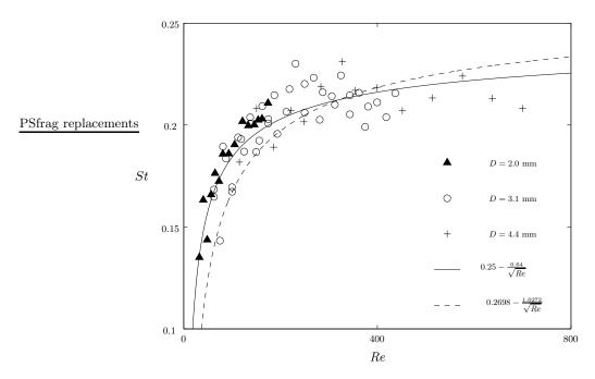
FIG. 4: Strouhal number as a function of the Reynolds number: measurements (symbols), best fit in a series in  $1/\sqrt{Re}$  (continuous line) and fit introduced in Ref. [23] (dashed line)
