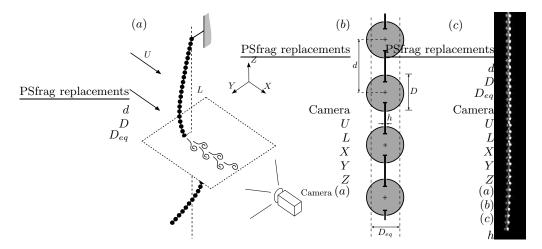
FIG. 1: (a) Experimental setup of the hanging string subject to a transverse flow. (b) Geometry of the chains that were used to model a string of equivalent diameter  $D_{eq}$ . (c) Visualization of Chain 3 during one typical experiment.
