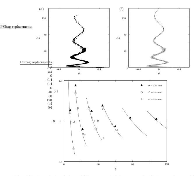
FIG. 5: Self-similarity of the mode shapes. (a) Superposition of all the experimental mode shapes as a function of the rescaled spanwise coordinate. (b) Comparison between the experimental mode shapes (grey) and the prediction of the linear model in section V (black continuous line). (c) Evolution of the self-similarity coefficient  $\kappa$  with the dimensionless length of the hanging string  $\ell$ , obtained from the experimental data (symbols) and using the linear model (continuous line)
