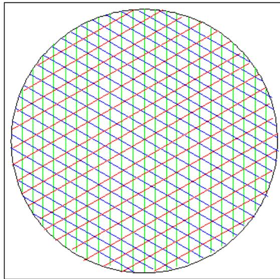
Figure-2 Diagram of the multiplexed holographic gratings for three primary colors
