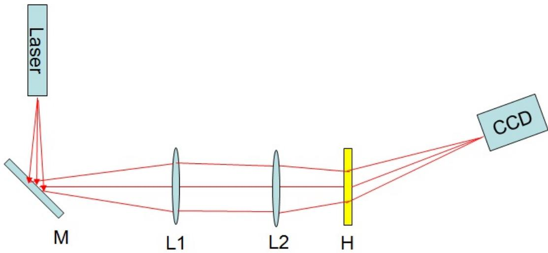
Figure-6 Setup for measuring spherical aberration of the 3 CCD imaging system.
