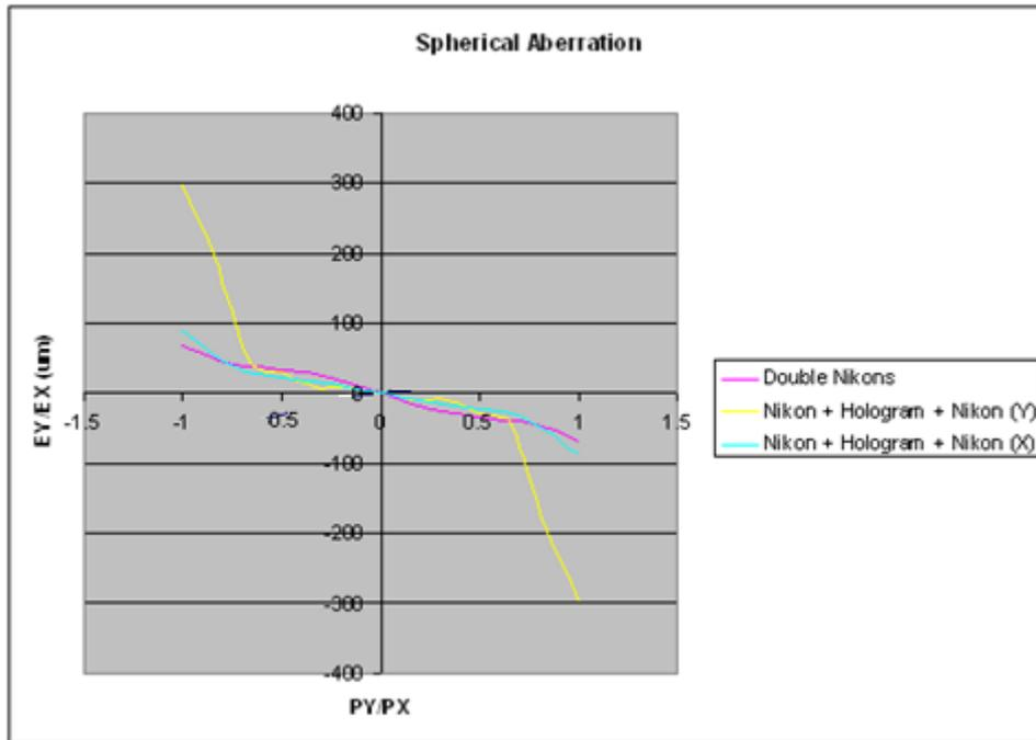
Figure-7 Spherical aberration plot of single lenses and the whole system
