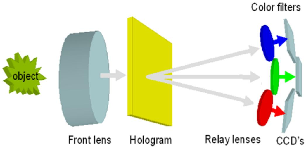
Figure-5 The 3 CCD imaging system based on multiplexed volume gratings.
