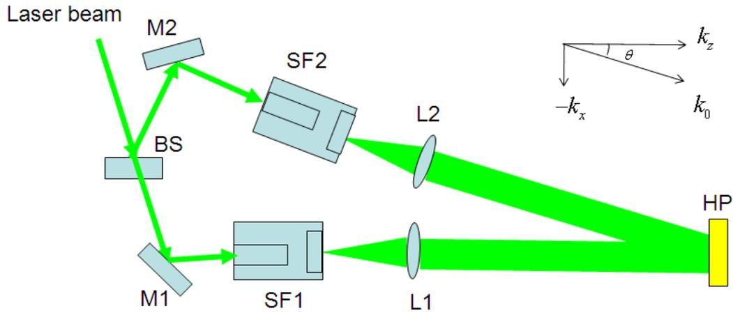
Figure-1 schematic diagram of writing the holographic gratings.
