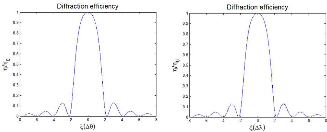
Figure-4 Diffraction efficiency for incident angle deviated from the Bragg angle.
