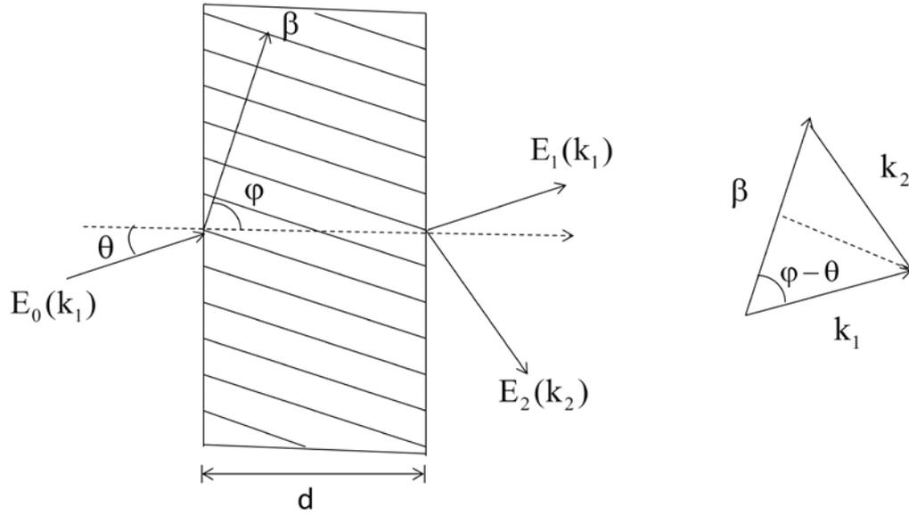
Figure-3 Block diagram of light diffracted by a thick hologram grating with slanted fringes.
