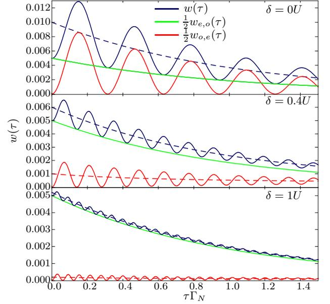
Figure 2. The waiting time distributions  $w_{e,o}(\tau)$ ,  $w_{o,e}(\tau)$ , and  $w(\tau)$  for  $\delta = 0U, 0.4U, 1U$ . For ease of visualization,  $w_{e,o}(\tau)$ ,  $w_{o,e}(\tau)$  have been multiplied by a factor 1/2. For comparison, the dashed curves for  $w_{o,e}(\tau)$  and  $w(\tau)$  are computed without the inclusion of the off-diagonal elements of the reduced density matrix between the Andreev bound states. Parameters:  $\Gamma_N = 0.01U$  and  $\Gamma_S = 0.2U$ .
