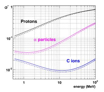
FIG. 4: Quenching factors for protons, alpha particles and carbon ions obtained from the eq. 3 using the best fit parameter  $kB=0.0125~g~cm^{-2}MeV^{-1}$  for LVD-scint (solid lines) and  $kB=0.0140~g~cm^{-2}MeV^{-1}$  for LVD-Gd (dashed lines).
