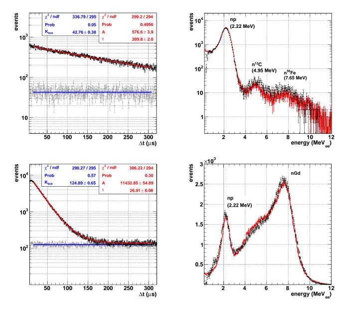
FIG. 1: Distribution of the absolute value of the time difference between the trigger and pre- or post-trigger in the same event (blu points) compared with the background level (in gray). Shapes are, as expected, flat for the background (fit function:  $y = k_{bck}$ ) and exponential for the data with the neutron source (fit function:  $y = Ae^{-t/\tau} + k_{bck}$ ). Top and bottom panel are relative to LVD-scint and LVD-Gd scintillator respectively.
