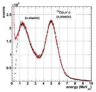
FIG. 3: Energy spectrum of the prompt signals after background subtraction (in black), compared with the simulation (in red). The detection threshold is at about 0.8 MeV $_{ee}$ . The value of the Birks factor which minimize the  $\chi^2$  is  $kB=0.0125~g~cm^{-2}MeV^{-1}$  for LVD-scint (top panel) and  $kB=0.0140~g~cm^{-2}MeV^{-1}$  for LVD-Gd (bottom panel).
