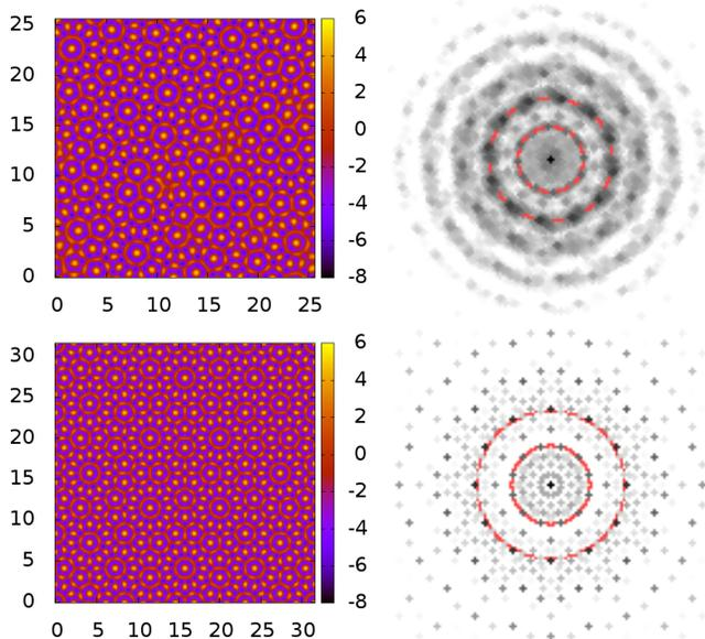
FIG. 5: Left:  $\ln[R^2\rho(\mathbf{r})]$  from DFT, for  $(\rho_0 R^2, A) = (3.5, 0.8)$ . Right: the corresponding Fourier transforms. The 12-fold symmetry is indicative of QC ordering. The upper profile was obtained from random initial conditions, while the lower one was started from initial conditions with QC symmetry.
