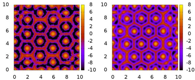
FIG. 3:  $\ln[R^2\rho(\mathbf{r})]$  for a system of  $N = 600$  particles with  $(\rho_0 R^2, A) = (4.0, 0.8)$  confined in a square region of side  $L = 10R$  obtained from BD simulations (left panel) and DFT (right panel). The system forms crystal A with a density profile consisting of an array of peaks surrounded by a connected network within which the particles are free to move – the CL state.
