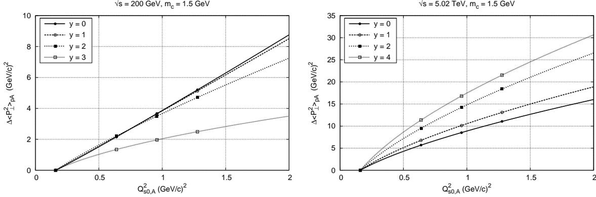
Figure 16: Mean transverse momentum square  $\Delta\langle P_{\perp}^2\rangle_{pA}$  of  $J/\psi$  as a function of  $Q_{s0,A}^2$  at  $\sqrt{s} = 200$  GeV (left) and  $\sqrt{s} = 5.02$  TeV (right). Fit with a form  $a[(Q_{s0,A}^2/Q_{s0,p}^2)^\alpha - 1]$  is also shown.
