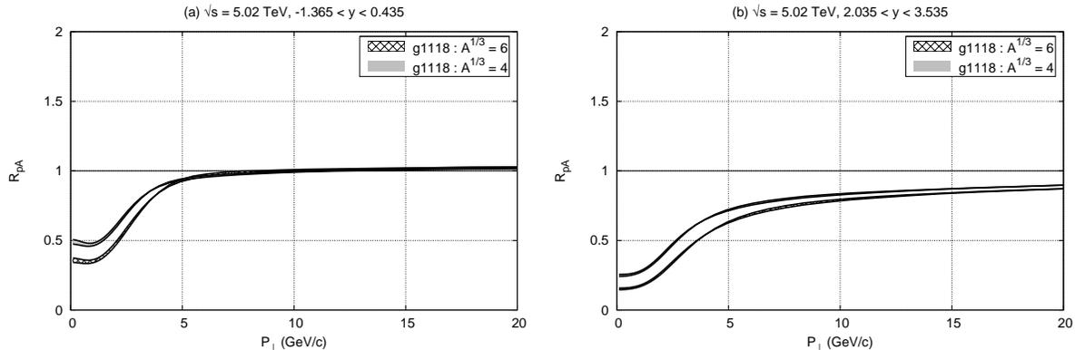
Figure 9: Initial-scale dependence of the ratio  $R_{pA}(P_{\perp})$  for  $J/\psi$  at (a) mid- and (b) forward-rapidities at  $\sqrt{s} = 5.02$  TeV.  $Q_{s0,A}^2$  is set to  $4Q_{s0,p}^2$  (upper) and  $6Q_{s0,p}^2$  (lower).
