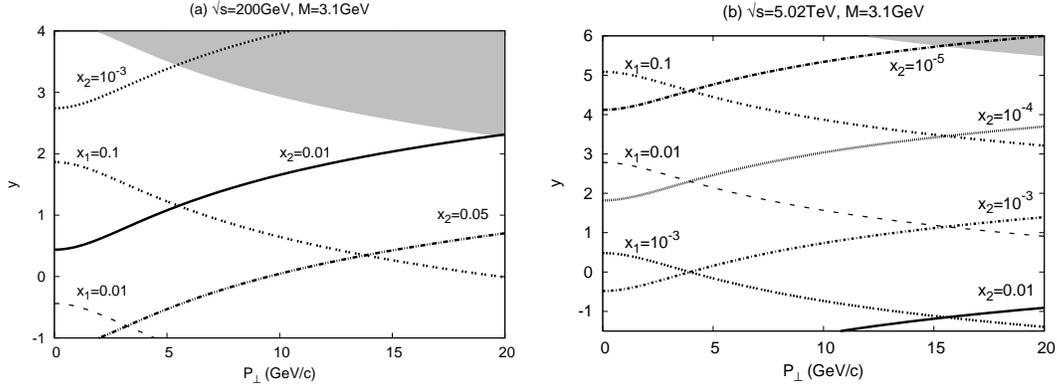
Figure 2: Kinematical coverage of the pair production in the plane of rapidity  $y$  and transverse momentum  $P_{\perp}$  for invariant mass  $M = 3.1$  GeV at (a)  $\sqrt{s} = 200$  GeV and (b)  $\sqrt{s} = 5.02$  TeV. Shown are the curves of constant  $x_{1,2} = (\sqrt{P_{\perp}^2 + M^2}/\sqrt{s})e^{\pm y}$ . The shaded region is kinematically forbidden.
