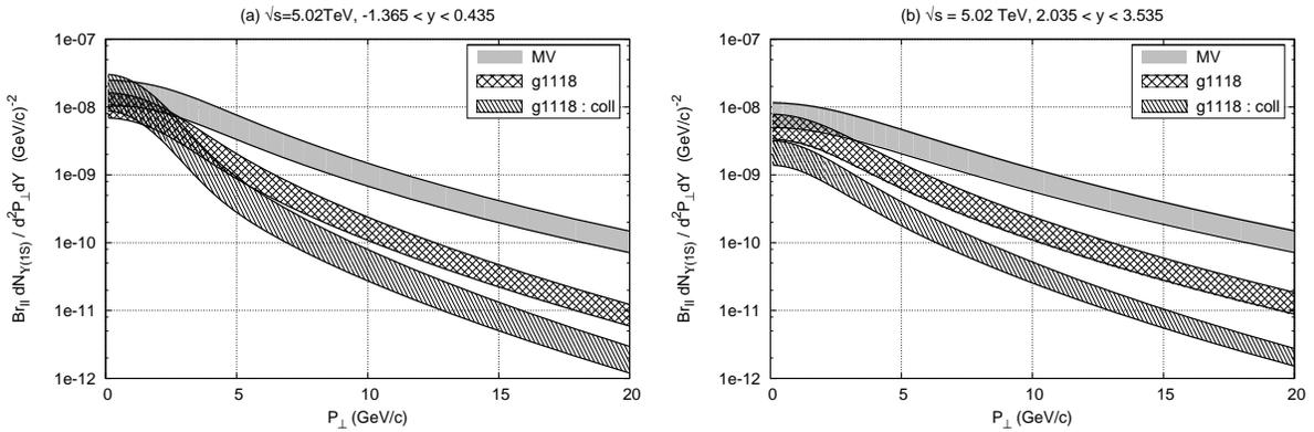
Figure 11: Transverse momentum spectrum of  $\Upsilon(1S)$  in di-lepton channel in pA collisions at  $\sqrt{s} = 5.02$  TeV for (a)  $-1.4 < y < 0.4$  and (b)  $2 < y < 3.5$ . Notations are the same as in Fig. 3.
