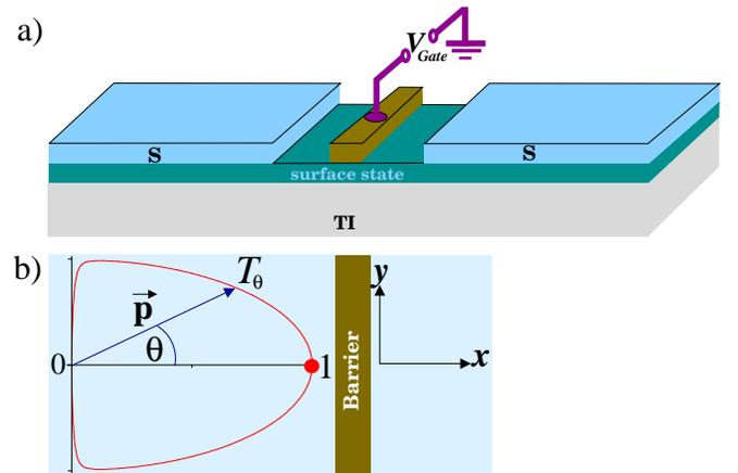
FIG. 1: (a) Schematic of S/TI/S junction with gated-induced barrier in the middle (see also text). (b) Scattering geometry in junction plane and polar plot of barrier transparency  $T_\theta$  as function of incidence angle  $\theta$  [see Eq. (31)].
