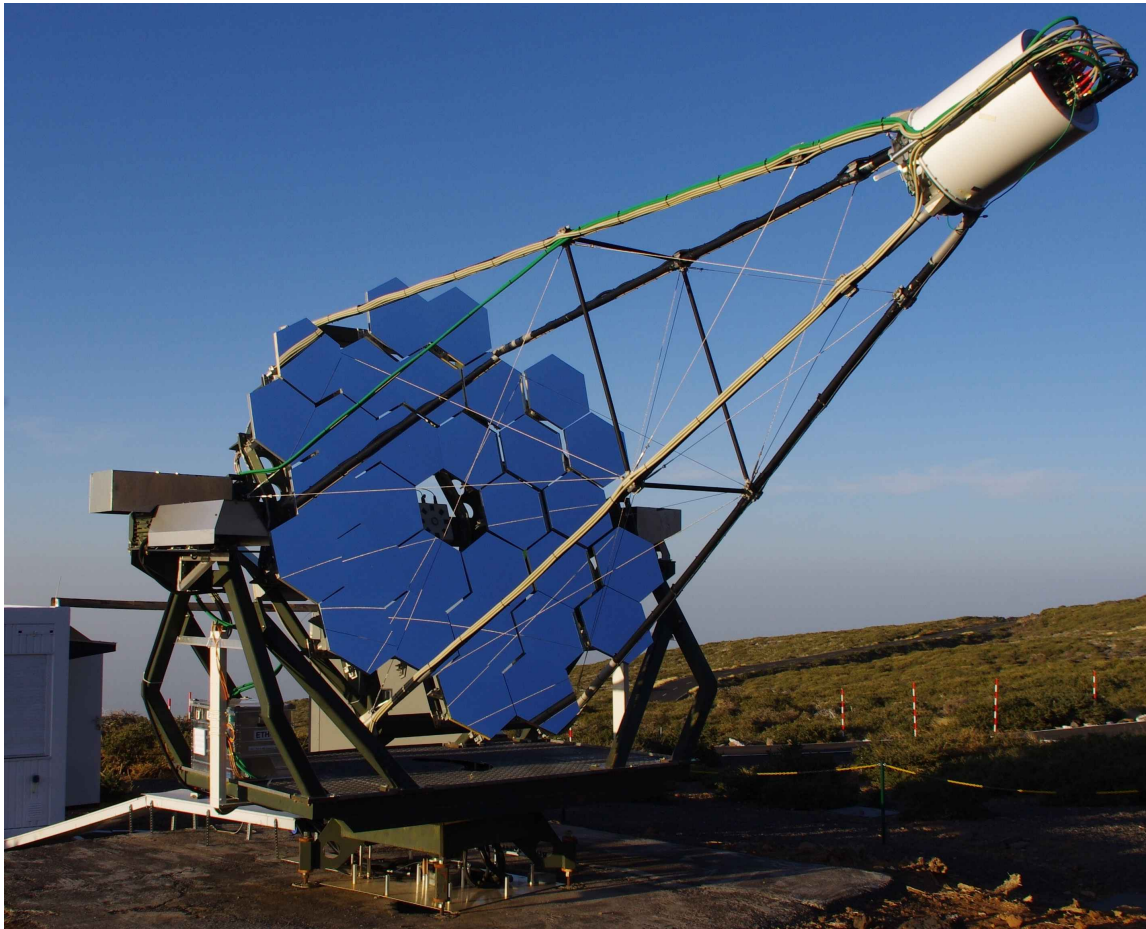
Figure 1. Photograph of the FACT telescope at the Observatorio del Roque de los Muchachos on La Palma (Canary Islands, Spain). At the top right the camera is visible (white cylinder), including the cables for power and communication connected at its back. The cables are fixed along the telescope masts and, together with the cables for the drive system, guided through a cable duct to the counting house (the container at the left). In the middle of the reflector where one mirror is missing, the light pulser and the video-camera are installed. The cooling unit is inside the metal box placed on the telescope platform.
