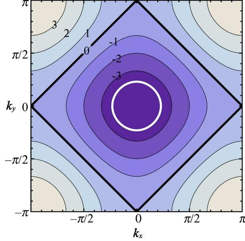
Fig. 2. (Color online) Dispersion surface  $E$  of a square coupled-cavity lattice system in the first Brillouin zone. The frequency of the contours are labeled with values of  $(E - \omega)/\kappa$ . The white contour indicates the operating frequency used to simulate the effective point source in Fig. 3(a). The black contour indicates the operating frequency used to simulate the beam source in Fig. 3(c).
