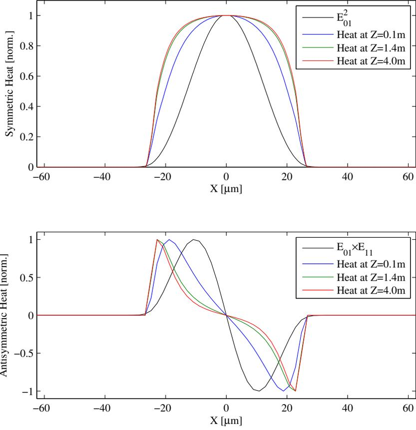
Fig. 4. Normalized symmetric part of the heat profile (upper plot) and antisymmetric oscillatory portion of the heat profile (lower plot) for the same counter-pumped fiber at the same three  $z$  locations indicated in Fig. 2. The oscillatory anti symmetric heat profile never closely matches the product of the fields of  $LP_{01}$  and  $LP_{11}$ .
