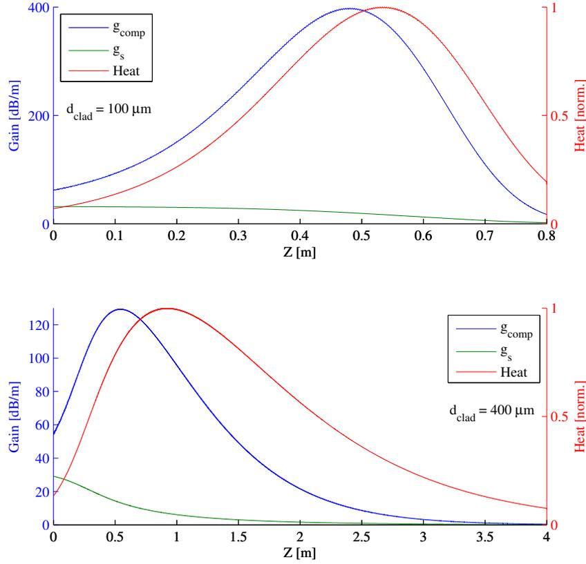
Fig. 6. Plots of laser gain  $g_s$ , total gain  $g_{comp}$  and heat versus  $z$  for the same co-pumped fibers and the same operating conditions as in Fig. 5. The upper plot is for a  $100 \mu\text{m}$  diameter cladding; the lower plot is for a  $400 \mu\text{m}$  diameter cladding. In both plots it is clear that the gain and heat profiles are not closely matched.
