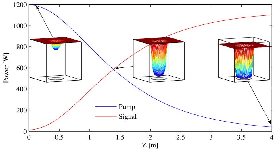
Fig. 1. Signal and pump powers versus  $z$  for co-pumped fiber with  $d_{\text{core}} = d_{\text{dope}} = 50 \mu\text{m}$ ,  $d_{\text{clad}} = 400 \mu\text{m}$ , operating at the mode instability threshold. The inset figures show the upper state fraction  $n_u$  profiles at  $z = 0.1, 1.4,$  and  $4.0$  m. The range of the  $n_u$  axis is 0-0.5. The circles on the bottom faces of the frames indicate the edge of the core.
