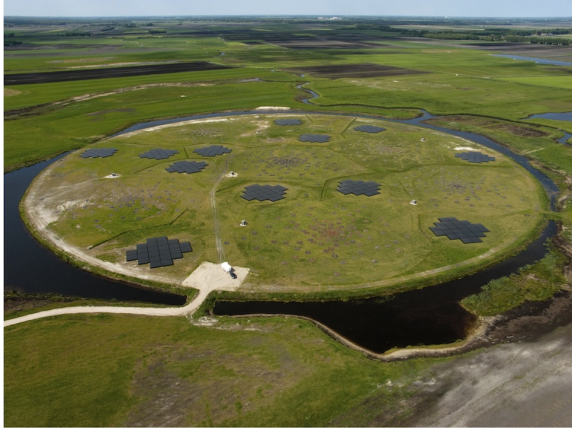
Figure 1: The central part of the LOFAR core. On the so called Superterp an area of about 0.1 \text{ km}^2 is populated with about 600 low-band antennas and 300 high-band antennas.
