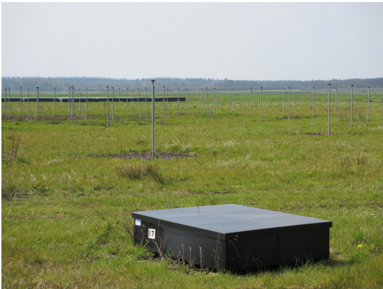
Figure 2: Impression from the LOFAR core. In the foreground a particle detector unit is shown. Behind it are the dipoles of the low-band antennas from one station. The black boxes in the background house the high-band antennas.
