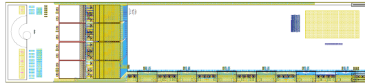
Figure 4: Layout of a PXD half-ladder. The white large area corresponds to the sensitive area, populated with 768 \times 256 DEPFET pixels. The area below the sensitive area contains the six Switchers and left of the sensitive area the DCDB and the DHP can be found.
