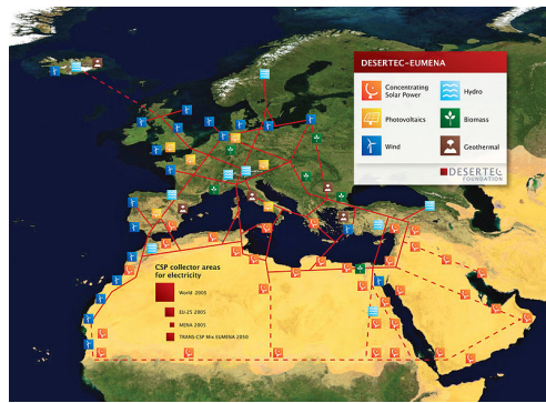
Figure 3. DESERTEC EU-MENA Map: Sketch of possible infrastructure for a sustainable supply of power to Europe, the Middle East and North Africa. The red dashed squares represent the total surfaces needed for solar collectors plants to cover the current electricity demands for the world [45].
