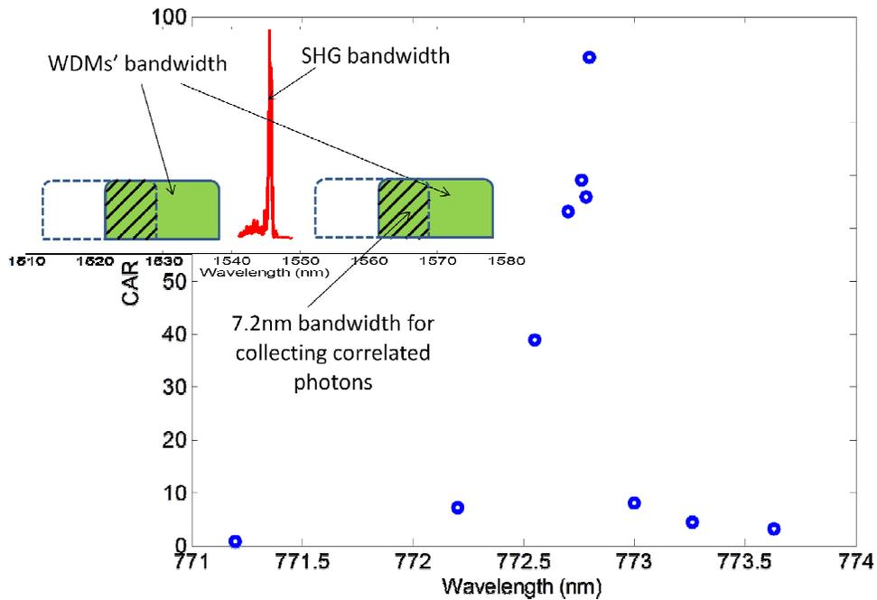
Fig. 4. Pump detuning. Figure inset: shows spectral location of collected pair photons (hatch pattern)
