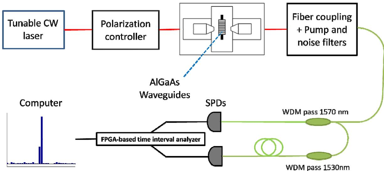
Fig. 2. Schematic of the setup for coincidence measurement in QPM AlGaAs superlattice waveguides.
