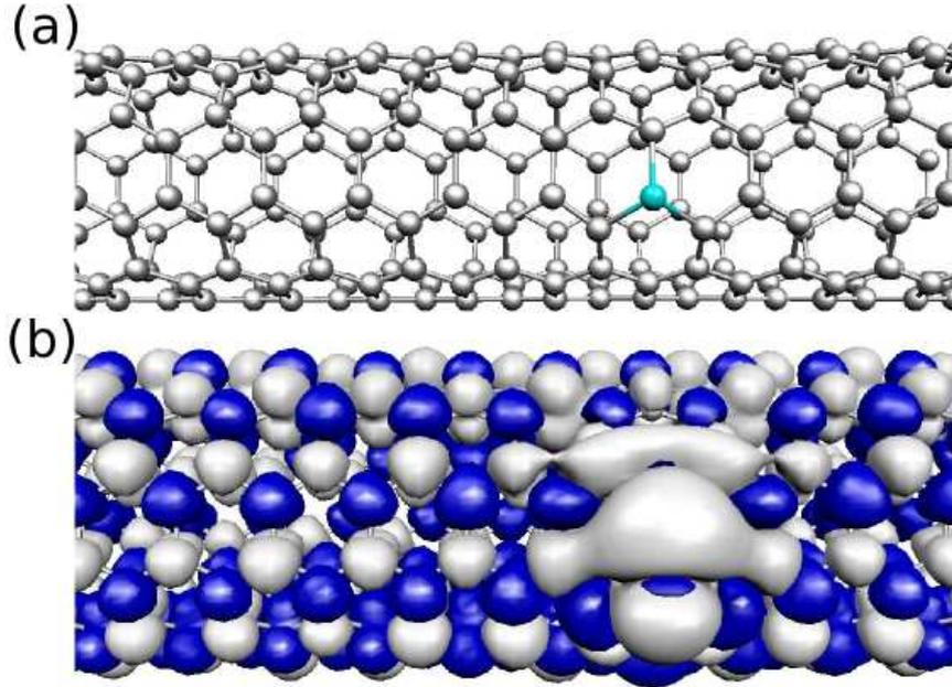
**Fig. 10** (a) Relaxed geometry of a substitutional Ni ( $\text{Ni}_{sub}$ ) impurity in a (5,5) SWCNT, and (b) isosurface ( $\pm 0.002 e^-/\text{Bohr}^3$ ) of the magnetization density with light (gray) and dark (blue) surfaces corresponding, respectively, to majority and minority spin. Adapted from (Santos et al. 2008).
