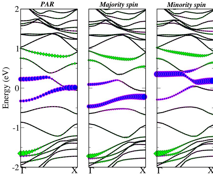
**Fig. 11** Band structure of a (5,5) nanotube containing a  $\text{Ni}_{sub}$  impurity in four unit cells for (left panel) a paramagnetic calculation (PAR), and for (middle panel) majority and (right panel) minority spins. Circles and diamonds correspond respectively to the amount of Ni  $3d_{yz}$  and  $3d_{xz}$  character. X-axis is parallel to the tube axis and y-axis is tangential. Adapted from (Santos et al. 2008).
