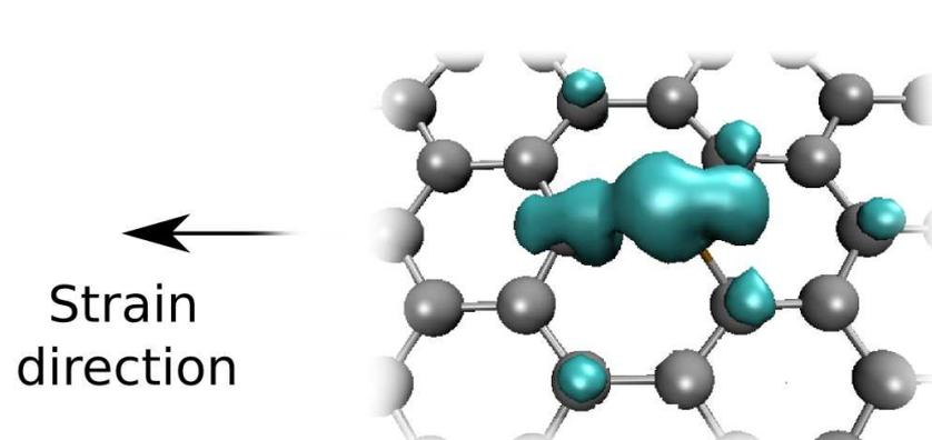
**Fig. 8** (a)-(b) Spin densities for  $\text{Ni}_{sub}$  defects at strains of 5.30% and 7.26% along the  $(n, n)$  direction. The strain direction is marked by the arrows in both panels. The isovalue cutoff at (a) and (b) panels is  $\pm 0.035$  and  $\pm 0.060 e^-/\text{Bohr}^3$ . Adapted from (Santos et al. 2012a).
