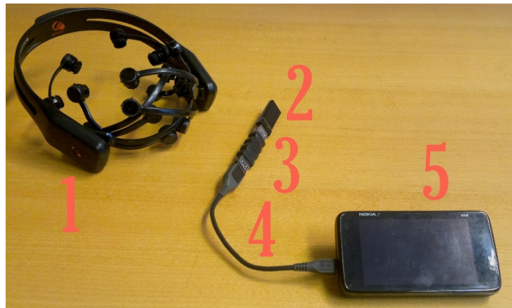
Figure 2. The system with Emotiv EPOC wireless EEG headset (1), Receiver module with USB connector (2), USB connector and adapter (3+4), and Nokia N900 (5).
