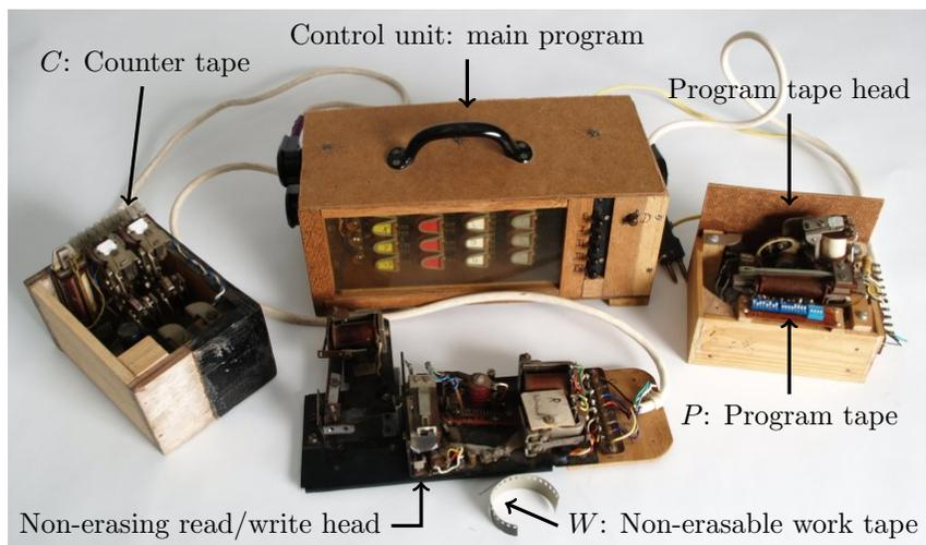
Figure 1: Hasenjaeger's universal electromechanical Turing machine. The wiring in the control unit encodes a universal program, that uses only four states and two symbols, for simulating Wang B machines. The program of a Wang B machine may be stored on the program tape. There are two additional tapes which are used for the simulation, a counter tape and a work tape.
