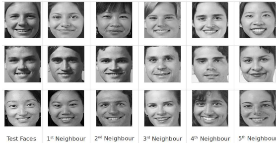
Figure 7: Exemplar correctly classified faces along with their 5 nearest neighbors. Obtained using 133 DCT coefficients with 5-NN classifier.
