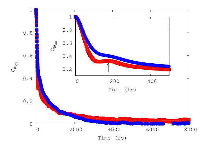
Figure 5: OH stretch frequency-frequency time correlation of OH groups initiated in H-bonded state (red) and those in non-bonded state (blue). The inset shows the short-time behaviour revealing a bump at 175 fs especially for the H-bonded OH groups. The short time behaviour shows a rapid loss of frequency correlation with a timescale of  $60\pm 5$  fs. Notice that while the blue end is slow at short times, the red end is slow at longer times.
