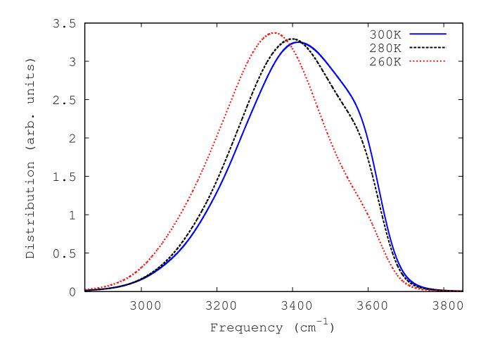
Figure 1: The OH-stretch frequency distribution obtained using the wavelet transform approach of Mallik *et al.*<sup>13</sup> for bulk water at temperatures of 260 K, 280 K and 300 K. Because of the 6% underestimation of the line centre at 300 K (with respect to the experimental value<sup>32</sup> of about 3400 cm<sup>-1</sup>), the frequency axis has been rescaled by a factor of  $1.06.^{32}$
