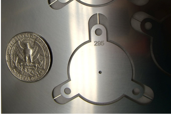
Figure 3: Photo of electrode #295 (Quarter for scale). The electrodes were photo-etched in a stainless-steel sheet and numbered individually. Prior to its assembly the electrode was held in place by ‘legs’ extending from the three equally spaced latches used to mount the electrode. These legs are cut off during installation.
