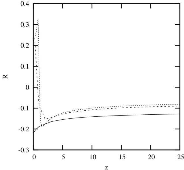
Figure 1: The scalar curvature  $R$ , in units of  $\lambda^3 V^{-1}$ , as a function of the fugacity  $z$  at  $D = 3$  and constant  $\beta$  for the cases of  $M = 1$  (solid line),  $M = 5$  (dashed line) and  $M = 25$  (dotted line).
