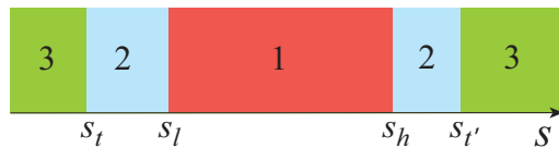
FIG. 2: (Color online) The schematic representation of the regimes observed for the different values of the observation time scale s : 1 — synchronous dynamics, 2 — intermittent behavior, 3 — asynchronous behavior. The coupling strength between oscillators is supposed to be fixed
