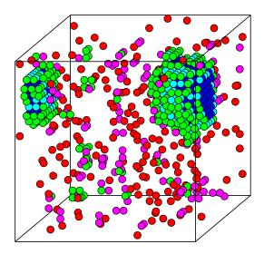
FIG. 1: (Color online). A snapshot taken from our Monte Carlo simulation of the 3D Ising model at  $T = 0.6 T_c$  and h = 0.30, showing a cluster of n = 685 up spins, i.e., close to the critical size for that h. Up spins are differently colored according to the number of nearest-neighboring up spins (blue, 6; cyan, 5; green, 2-4; magenta, 1; red, 0). Down spins are not shown.
