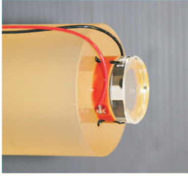
Figure 1: Picture of the cavity with PZT stack actuator attached between spacer and mirror via a three point glue joint on each side (black spots).
