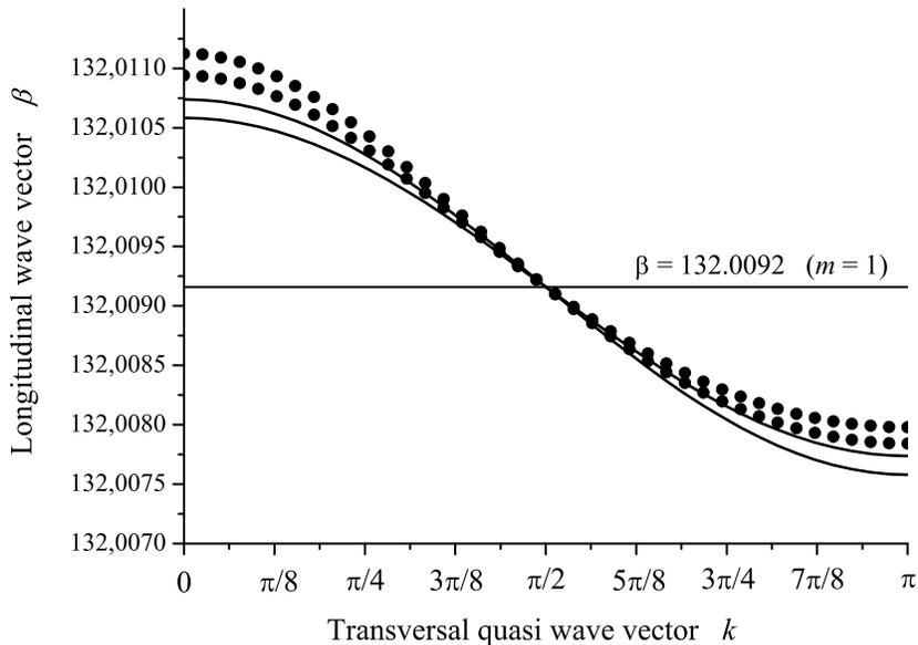
Figure 4: Isofrequency curves originating from the propagation constant  $\beta = 132.0092$  ( $m = 1$ ). Dots for the curves obtained by MMSF, solid lines for the curves obtained by phenomenological model.
