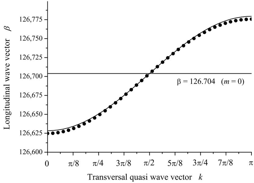
Figure 2: Isofrequency curve originating from the propagation constant  $\beta = 126.704$  ( $m = 0$ ). Dots for the curve obtained by MMSF, solid line for the curve obtained by phenomenological model.
