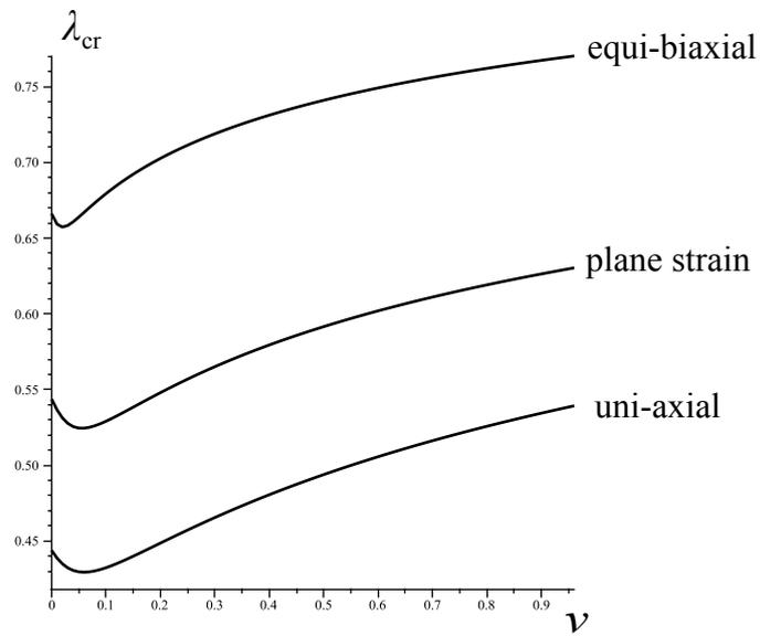
Figure 3: Surface instability of a compressed solid with strain-energy density given by (1). For uni-axial compression, plane strain compression, and equi-biaxial compression, the surface instability occurs earlier than for the neo-Hookean solid (which corresponds to  $\nu = 0$ ), once  $\nu > 0.15$ .
