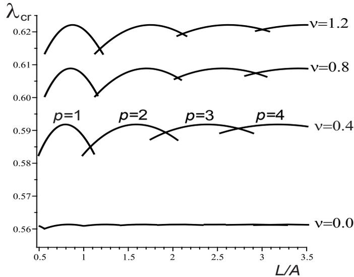
Figure 6: Bending instability for a rectangular block with length-to-depth ratio  $L/(2A) \in [0.25, 1.75]$ . The neo-Hookean solid ( $\nu = 0.0$ ) can be bent more than solids with strain energy density (1), see plots at  $\nu = 0.4, 0.8, 1.2$ .
