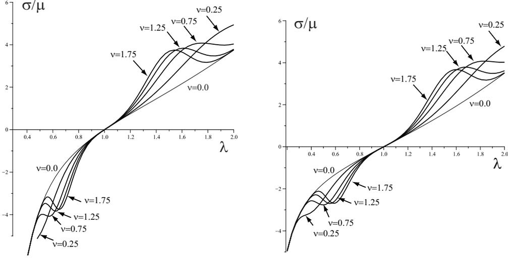
Figure 1: Effect of localized strain softening for the large deformations of solids with strain-energy density given by (1). Stress-stretch curves in compression ( $\lambda < 1$ ) and in tension ( $\lambda > 1$ ), for plane strain deformation (figure on the left) and uni-axial deformation (figure on the right), with  $\nu = 0$  (neo-Hookean solid), and  $\nu = 0.25, 0.75, 1.25, 1.75$ .
