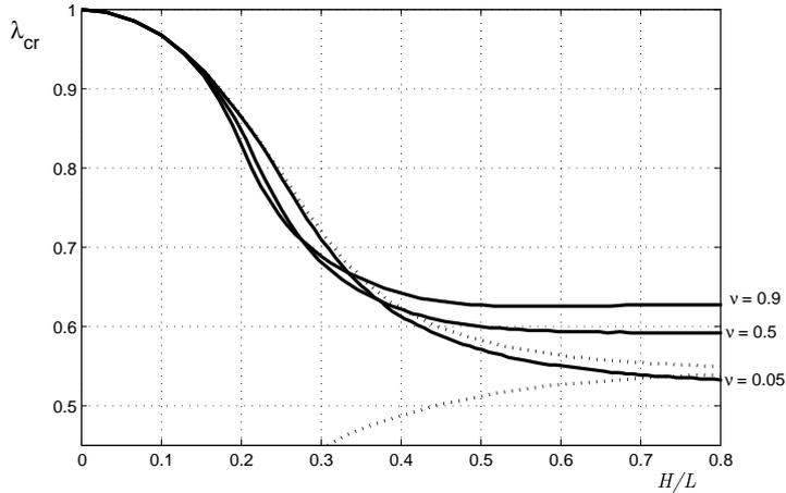
Figure 4: Buckling of a compressed slab in plane strain: critical stretch against  $H/L$ , the slab's initial slenderness. Solid curves: solids with strain-energy density given by (1). Dashed curves: neo-Hookean solids.
