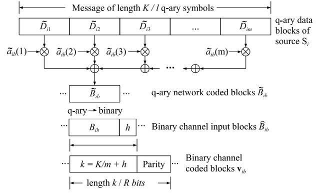
Fig. 2. A source  $S_i$  divides its message of length  $K$  bits into  $m$  blocks. RLNC over  $\text{GF}(q)$  is then used to create  $q$ -ary network coded blocks  $\tilde{B}_{ib}$ . After  $q$ -ary to binary conversion, a header of size  $h$  bits is appended to each block and the resulting block of size  $k = K/m + h$  bits is protected by a linear channel code of rate  $R$  to create binary channel coded blocks  $\mathbf{v}_{ib}$ .
