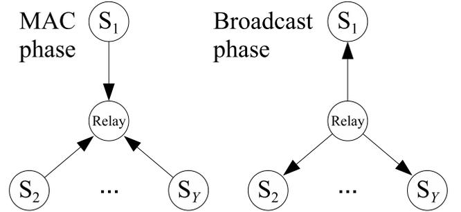
Fig. 1. Star network in which  $Y$  sources communicate over noisy BSCs with the help of a central relay.
