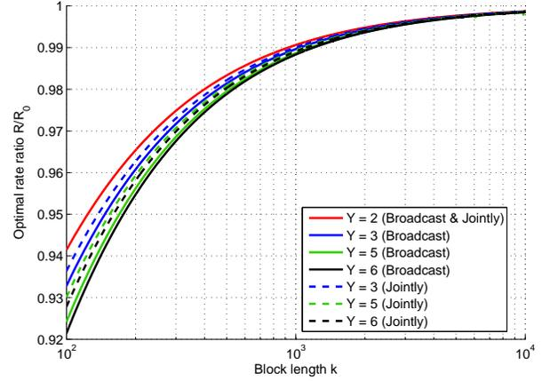
Fig. 7. Optimum channel coding rate  $R$  for broadcast (solid lines) and considering transmission to and from the relay jointly (dashed lines) as a fraction of the cutoff rate  $R_0$  for different channel input block lengths  $k$ .
