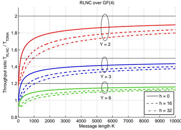
Fig. 10. Average throughput ratio  $T_{\text{RLNC}}/T_{\text{TDMA}}$  for GF(4).
