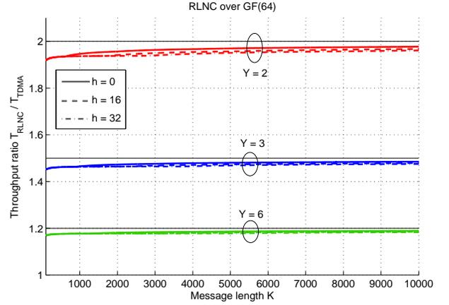
Fig. 11. Average throughput ratio  $T_{\text{RLNC}}/T_{\text{TDMA}}$  for GF(64).
