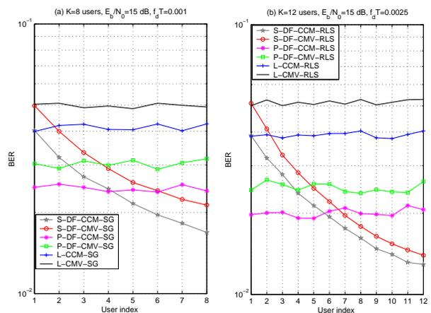
Fig. 9. Performance of the receivers in a fading environment in terms of individual BER versus user index for (a) SG and (b) RLS algorithms.
