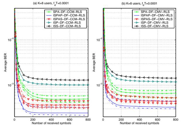
Fig. 6. BER convergence performance of RLS algorithms with iterative receivers for different numbers of parallel branches  $L$  at  $E_b/N_0 = 15$  dB in a slow fading environment (a) CCM (L=2 - dashed line, L=4 - solid line and L=8 - dash-dotted line) .
