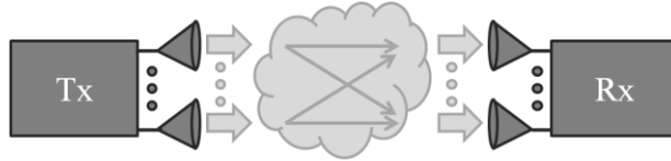
Figure 1.7 Multiple-input, multiple-output system
