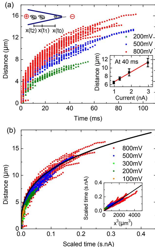
FIG. 3. (a) Tracks of multiple DNA molecules for three different voltages. The interval between successive frames is  $\Delta t = 1.98 \text{ ms}$ . The distance covered 40 ms from the start of translocation scales linearly with applied voltage (Inset). (b) The tracks for all voltages have been scaled and fitted with a model described in equations 4 and 5.
