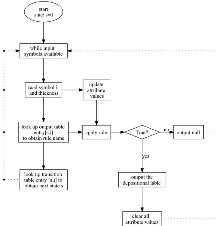
Figure 17: The operating procedure of the FST.
