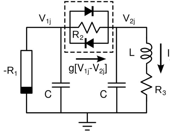
FIG. S1. **Chaotic electronic oscillator** with negative resistance  $-2,814 \Omega$ ,  $10 \text{ nF}$  capacitors,  $55 \text{ mH}$  inductor (dc resistance  $353 \Omega$ ) in series with resistance  $100 \Omega$ , and a passive nonlinear element (resistance  $8,067 \Omega$ , and back-to-back parallel diodes, type 1N914, dashed box).
