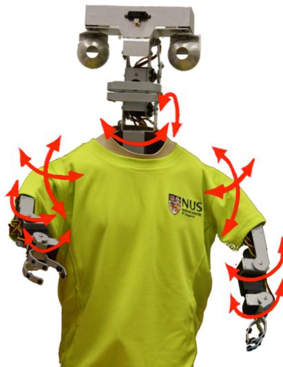
Fig. 1. The robot that was used to demonstrate the gestures. The arrows illustrate the 10 degrees of freedom of the robot.
