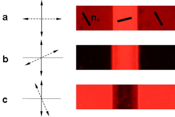
Figure 6: Microscopic images obtained at  $\varphi_p > 0$  for different orientations of the polarizer: (a) crossed polarizers; dark state orientation for the regions (b) outside and (c) within the interelectrode gaps.
