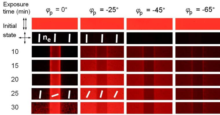
Figure 4: Microscopic images of the cell (filter with  $\lambda = 630$  nm was used) in crossed polarizers for LPUV irradiation at different exposure times for various values of the polarization azimuth. The interelectrode gap ( $g = 50 \mu\text{m}$ ) is indicated. The ac electric field is  $E = 2 \text{ V}/\mu\text{m}$  and the initial irradiation dose is  $D_p = 0.27 \text{ J}/\text{cm}^2$ .
