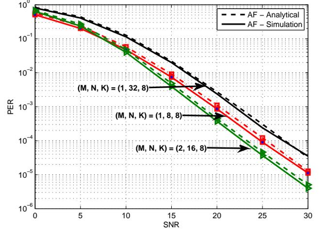
Fig. 4. Comparison of analytical and simulation results for AF with different values of the  $(M, K, N)$ .
