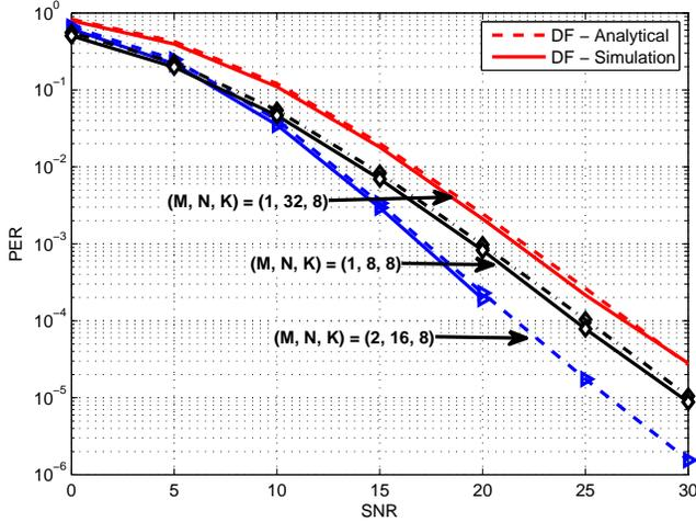
Fig. 5. Comparison of analytical and simulation results for DF with different values of the  $(M, K, N)$ .
