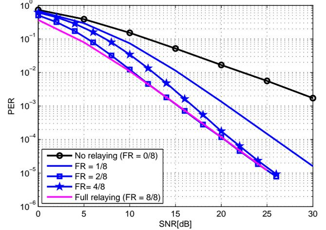
Fig. 7. PER for different forwarding rates FR with DF relaying.
