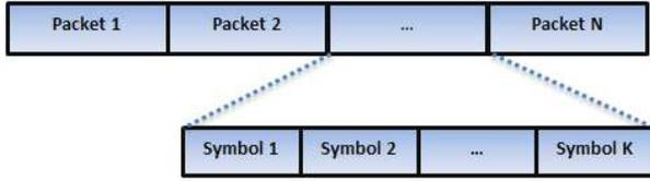
Fig. 2. Frame structure.
