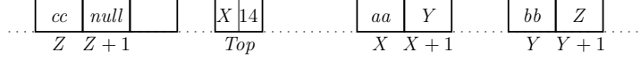
Figure 13: A state corresponding to abstract stack \langle aa, bb, cc \rangle , where \text{ptr}.(*\text{Top}) = X and \text{ctr}.(*\text{Top}) = 14
