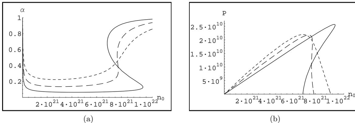
Figure 1:  $\alpha(n_0)$  and  $P(n_0)$  in the Debye-Hückel model at  $T = 20\,000$  K (—),  $T = 23\,000$  K (---), and  $T = 26\,000$  K (- - -).
