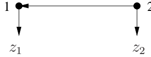
Fig. 5. The perturbed network consisting of a unidirectional link and normalized demands z_1 = e_1/\sigma_e , z_2 = e_2/\sigma_e .
