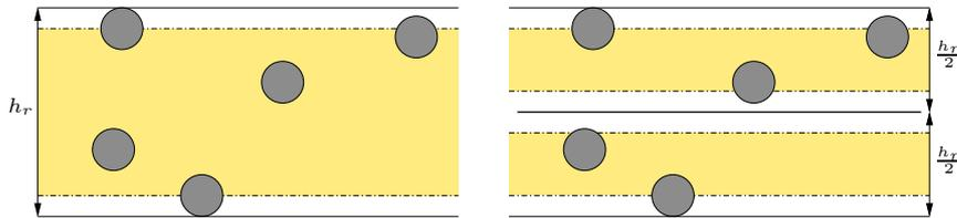
**Figure 6** Sketch of channel of width  $5\epsilon$  with and without an intermediate wall that creates two lanes. The domain available to the particles' centres' in each case is shaded in yellow. Left: one narrow channel with  $h = 4$ . Right: two narrow channels each with  $h = 1.5$  (roughly equal to  $h^*$  for maximal exclusion effects).
