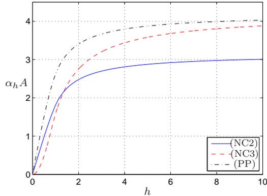
**Figure 4** Excluded volume  $\alpha_h A$  as a function of the confinement parameter  $h$  in three cases: two-dimensional channel (NC2) ( $A = h$ ), three-dimensional channel (NC3) ( $A = h^2$ ), and parallel plates (PP) ( $A = h$ ).
