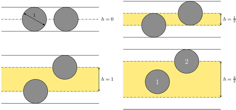
**Figure 3** Sketch of the channel domain (shaded in yellow) for different values of  $h$  with particles of diameter one (note that here we are depicting the actual particles, not their excluded-area which has *radius* one). Single-file channel for  $0 \leq h < 1$  (with  $h = 0$  being the extreme case in which particles can only move in the axial direction). When  $h = 1$  particles can *just* pass each other, and for  $h > 1$  (bottom row) particles can more easily change order.
