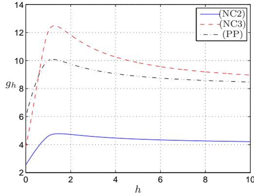
**Figure 5** Coefficient  $g_h$  as a function of the confinement parameter  $h$  in three cases: two-dimensional channel (NC2), three-dimensional channel (NC3), and parallel plates (PP).
