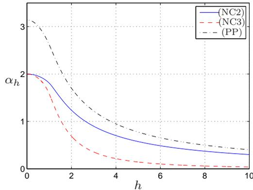
**Figure 2** Excluded-volume coefficient  $\alpha_h$  as a function of the confinement parameter  $h$  in three cases: two-dimensional channel (NC2) (11), three-dimensional channel (NC3) (12), and parallel plates (PP) (14).
