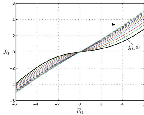
**Figure 12** Steady-state flux  $J_0$  versus tilt  $F_0$  from solving (25) for increasing values of  $g_h\phi$  (from 0 to 1). The coloured lines correspond to finite-size particles ( $g_h > 0$ ). The thick black line corresponds to point particles ( $g_h = 0$ ) as shown in Reimann (2002, Figure 2.4).
