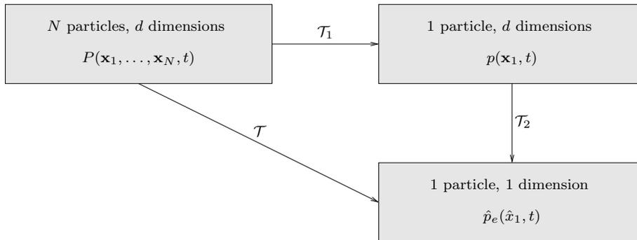
**Figure 1** Schematic of the problem solution steps for  $d_e = 1$  [narrow-channel cases (NC2) and (NC3)]. The goal is transformation  $\mathcal{T}$ , to obtain an effective one-dimensional equation along the channel for the marginal density of one particle. We achieve this with the combined steps  $\mathcal{T}_1$  followed by  $\mathcal{T}_2$ .
