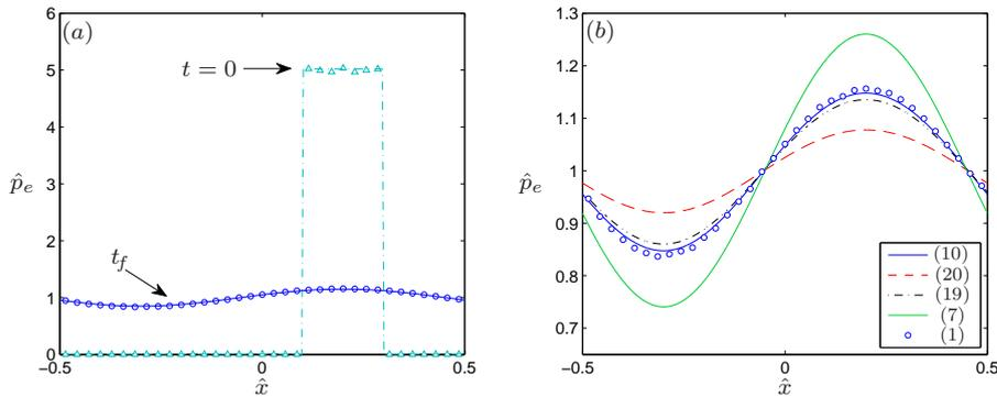
**Figure 8** One-dimensional density  $\hat{p}_e(\hat{x}, t)$  in a channel of width  $\epsilon h$  with periodic boundary conditions at  $\hat{x} = \pm 0.5$ : solution of the continuum model (10) for finite-size particles versus individual-based model simulations of (1) and limiting models (7), (19) and (20). Other details of the plots are given in the caption of Fig. 7. (Color figure online)
