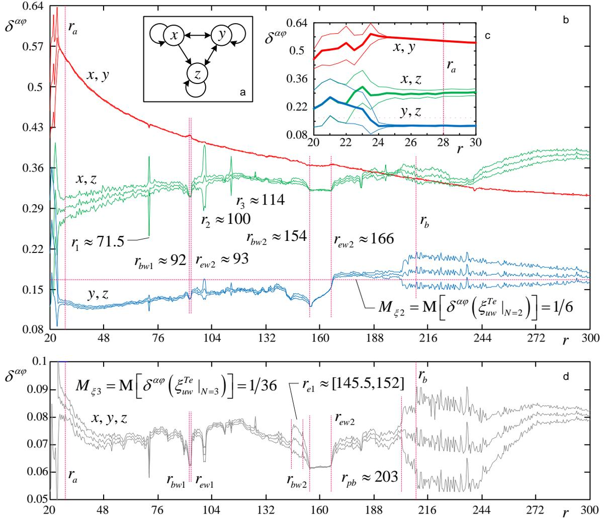
**Fig. 1.** Analysis of oscillations in model system (8): (a) schematic diagram of coupling between variables; (b, c) plots of coefficient  $\delta^{\alpha\varphi}$  vs.  $r$  for  $\mathbf{s}(t)$  sets with two components; (d) the same for  $\mathbf{s}(t)$  sets with three components. Confidence intervals are indicated for a probability of  $1 - \alpha$  ( $\alpha = 10^{-3}$ ); the reference sequence as formed in the alphabet  $T_e^{\alpha\varphi} = \{T3N, T3P, T5N, T5P, T6, T7\}$  (see [10]).
